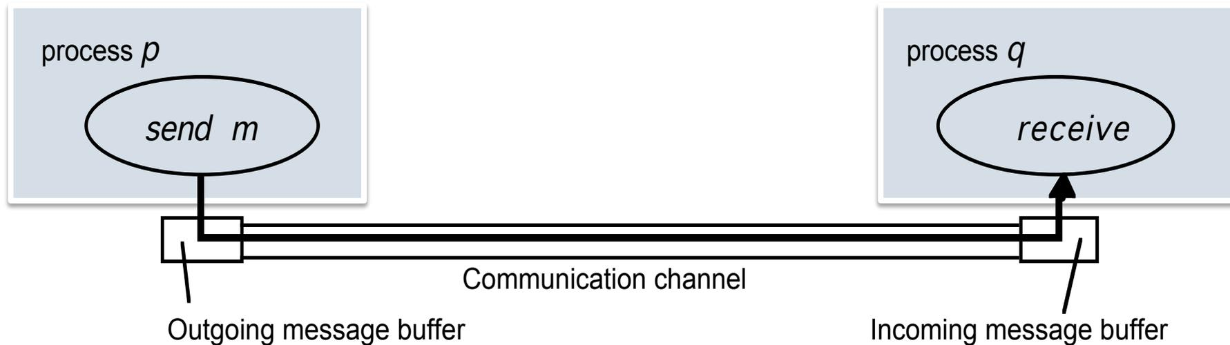
**Synchronous communication:** sending and receiving processes synchronize at every message = send and receive are blocking operation
